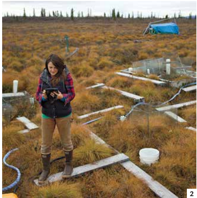
SENSORS in white chambers near the snow-capped Alaska Range measure the soil's uptake and release of carbon dioxide (1). Researcher Meghan Taylor of Northern Arizona University records the data (2).
